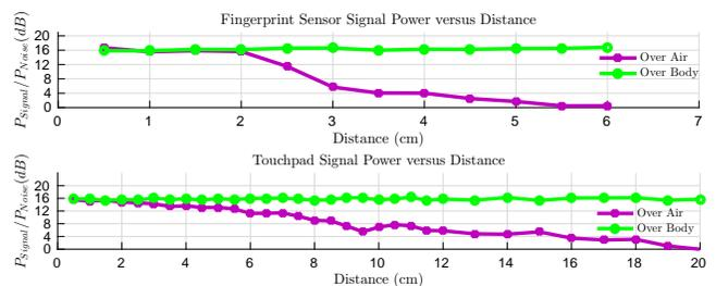
Figure 2: Comparing the strength of the EM signals
