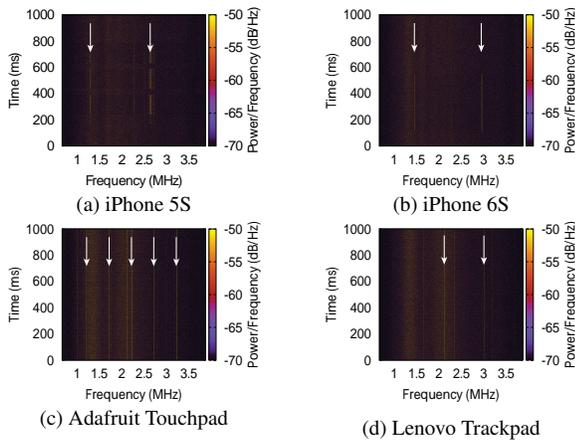
Figure 4: **Spectrograms of the four input devices.** The white arrows are shown in the graphs for emphasis.
