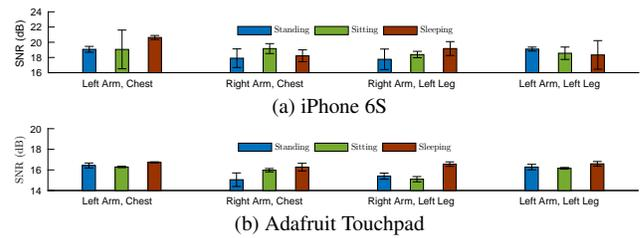
Figure 6: Signal strength for different body postures.
